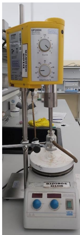
Figure V.7 UAE equipment: Hielscher UP200H sonotrode, jacketed reactor, electric plate with controlled heating and stirring
